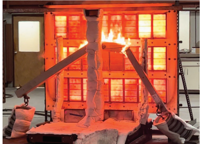
During testing conducted at the Western Fire Center in Kelso, WA, this composite fiberglass crossarm ignited after just 2½ minutes of exposure to radiant heat with no flames. Less than 30 seconds later it collapsed. A second composite crossarm crumpled less than 7 minutes into the test. A wood crossarm also ignited, but continued to support its load for the entire 30-minute test duration.
