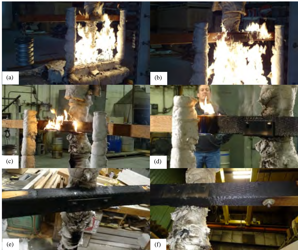
Figure 6. Images during Test 5 showing (a) burner on, (b) attached flames, (c) burner off, (d) continued flames, and (e-f) after test.
