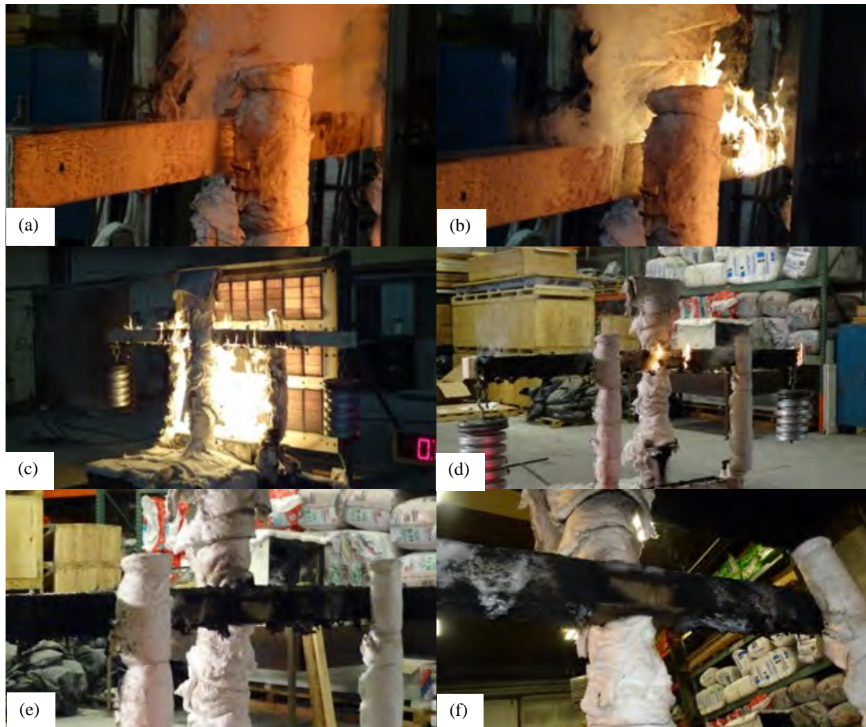
Figure 8. Images during Test 3 showing (a) darkened face, (b) ignition, (c) burner on, (d) burner off, and (e-f) after test.
