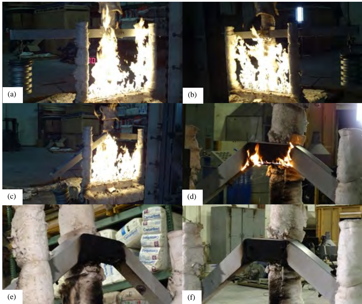
Figure 5. Images during Test 4 showing (a) burner on, (b) attached flames, (c) east collapse, (d) continued flames, (e) flames out, and (f) after test.
