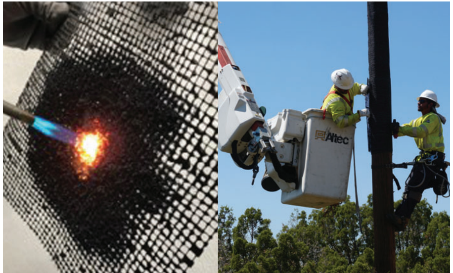
Fire wraps coated with intumescent polymers protect wood poles by creating an insulating layer that expands when exposed to heat. The wraps can be easily applied on new poles or around in-service poles.
