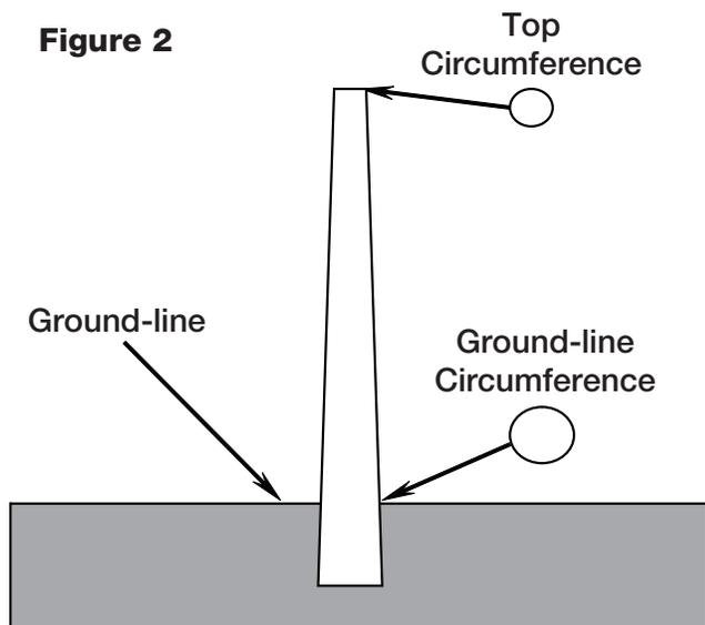
The 2017 NESC requires that wood structures be designed to withstand the specified loads in Rule 252 multiplied by the load factors in Table 253-1 without exceeding the permitted stress level at the
