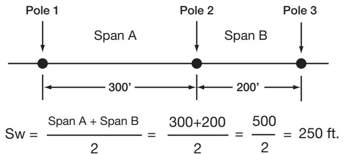
To determine the maximum transverse wind span for a given pole length and class with a set of specified conductors attached to a pole top assembly, the designer must calculate and sum the forces acting on the pole and wire with applied NESC strength and load factors.
