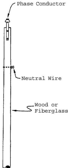
Figure 1. Typical rural distribution single-phase pole configuration, 7.2kV.
