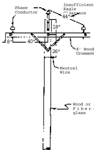
a 20-degree angle between the outer and center phase wire. This separation is appropriate in areas where large raptors are less likely to occur. Additional protection is required in areas with eagles and other large raptors.
