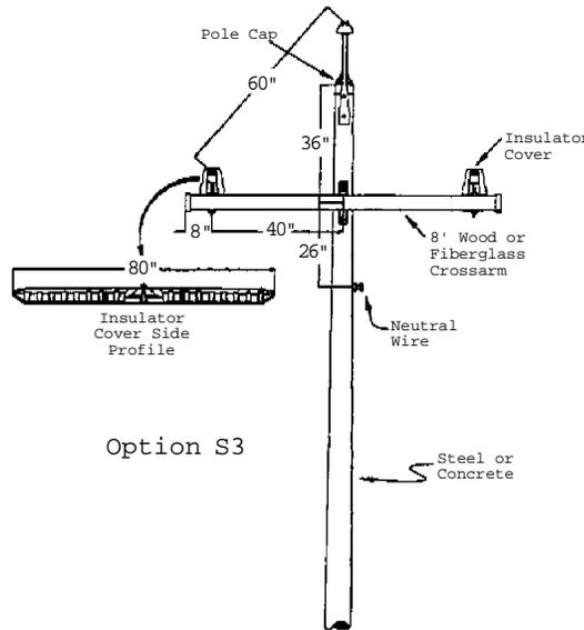
Figure 4 – Option S3. Three-phase steel/concrete pole configuration with Kaddas Bird Guards™, 7.2/12.47kV.
