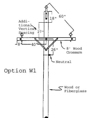
Figure 3. Typical rural distribution three-phase pole configuration, 7.2/12.47kV.
